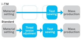
As the appropriate thread tension adjustment is applied regardless of the thread type, mass production can be started quickly.
