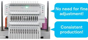
i-TM is mounted on the tension base in place of the previous tension knobs.
